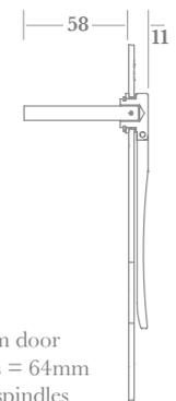
minimum door thickness = 64mm (shorter spindles available on request)
